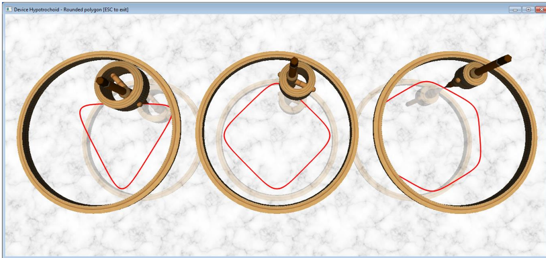
Figure 36. Triangle, square and hexagon as curtate hypotrochoidal polygons
